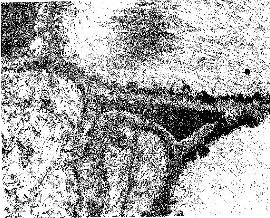
Fig. 5 Aragonite rims on micrite envelopes (dark grain coatings) cementing mollusc and bored coral sand grains. Field view is 1 mm. Crossed nichols.
