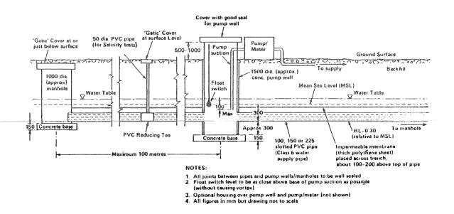
Figure 33. Cross-section through typical Home Island infiltration gallery.
