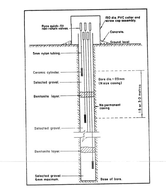
Figure 29. Borehole salinity monitoring system.
