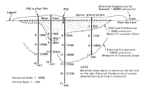
Figure 32. Cross-section through Home Island lens showing shape of lens at time of drilling in Oct/Nov 1987.
