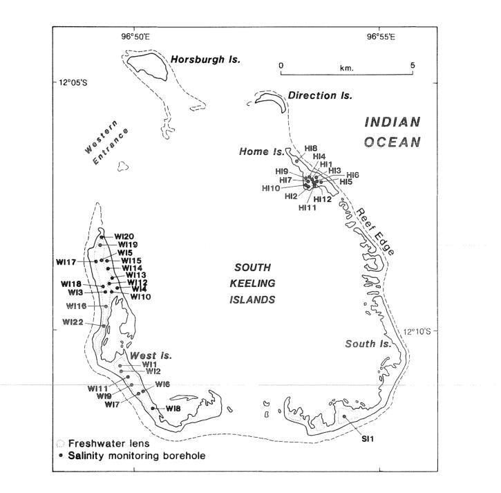
Figure 28. Location of Boreholes and freshwater lenses.
