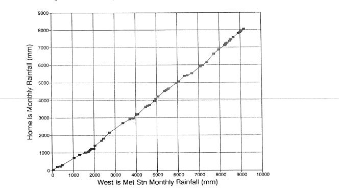
Figure 14. Double mass curve of monthly rainfall for the meteorological station and Home Island, 1987-1991.
