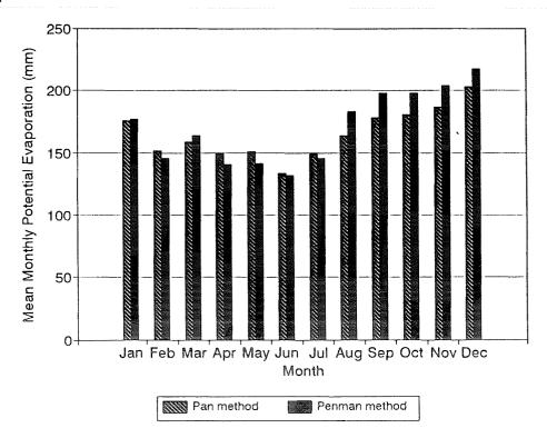
Figure 19. Mean monthly potential evaporation estimates using pan and Penman methods.
