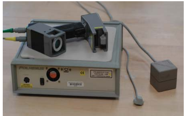
Figure 4: Scanner components (from left): processing unit with want on top, reference receiver and transmitter
