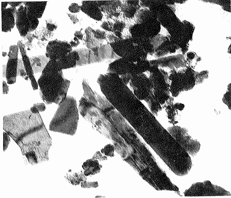
Figure 9: Electron photomicrograph of the fines ( <0.074\text{mm} ) from sample TA-8, showing whole and fragmented aragonite needles and laths. The prominent dark colored acicular crystal at lower right is between 1 and 2 microns in length.
