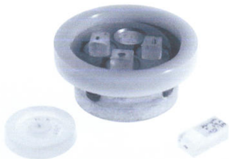
Fig. 2. Epoxy disc (left) and tablet (right) embedding forms, with holder for preparation and examination of four tablets. Preparation time is greatly reduced by mass production, but benefits are found in the application of principles to single samples (left).
