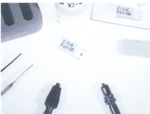
Fig. 4. Essential materials for embedding, with tablet with sample on shelf at center. Clockwise from top center: samples in vial, labeled half-tablets ready to mount samples, adhesive-backed label paper, needle holders with fishing-line probes, tweezers, commercial mold for final casting
