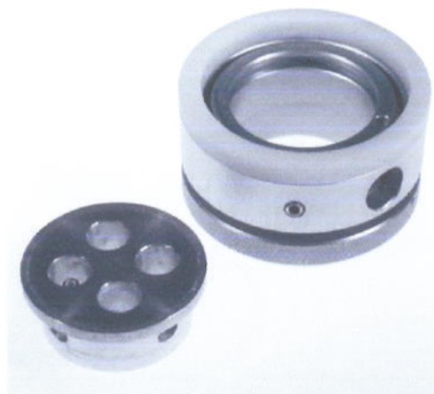
Fig. 11. Holder, without ring, can be used in Struers Accustop. This calibrated fixture (20 \mu\text{m} divisions) allows removal of measured amounts of material.
