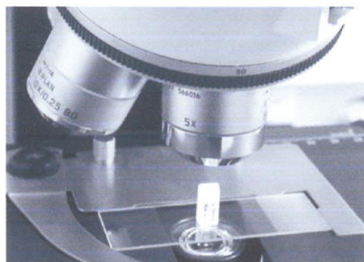
Fig. 8. Polished sample in tablet can be placed directly on stage for examination.
