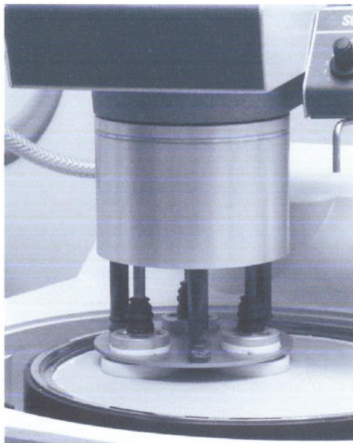
Fig. 18. Detail of Rotoforce-1 motorized sample mover. Pressure is controlled by adjustable air pressure pads over each holder. This head rotates at 60 rpm, while large platen rotates at adjustable speeds.
