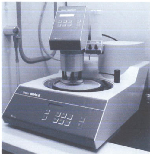
Fig. 17. Semiautomatic polisher (based on Struers RotoPol-15) for processing up to 12 samples in three holders simultaneously
