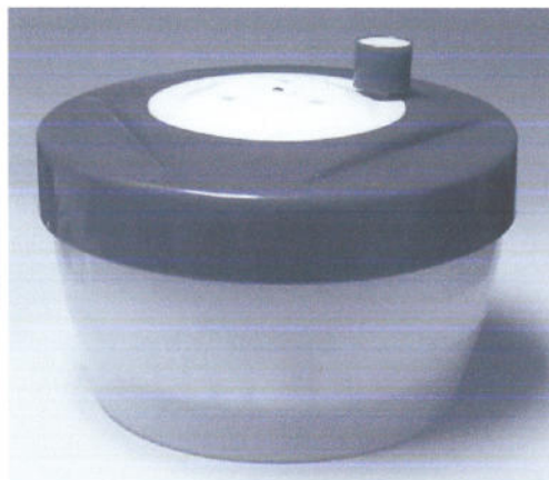
Fig. 24. Kitchen fruit and vegetable spinner serves as an inexpensive, highly effective centrifuge.
