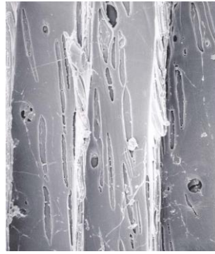
Scanning electron micrographs of soft-rotted wood from the King Midas tomb showing numerous holes within the cell wall in transverse section (right) and cylindrical cavities in radial section (left).
