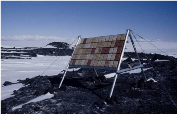
Fig. 5. One of three test racks to evaluate various wood treatments for potential use in protecting exterior woods of the historic huts.
