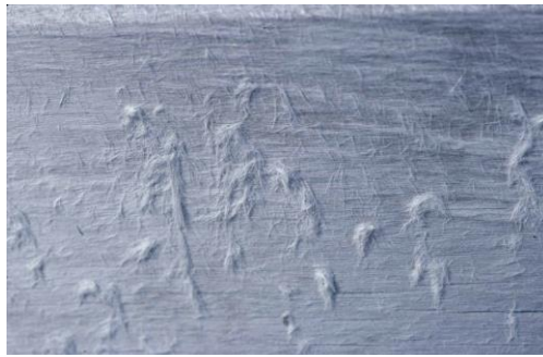
Exterior wood from Scott's hut at Cape Evans, Antarctica showing defibrillation caused by salts.
