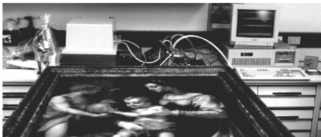
Fig. 1. The prototype Bomem–Michelson FTIR with ambient temperature 25-cm single-pass cell with a fixed path length optimized to measure CO 2 , vacuum pump, a computer for data reduction and analysis and control of the valving system.
