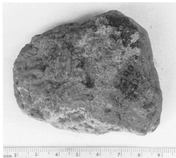
Fig. 9c. Crucible 13 showing powdery accretions and weathering products on the surface
