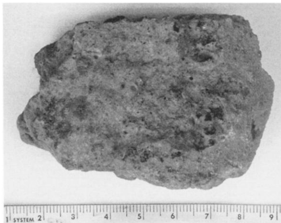
Fig. 9b. Crucible 4 showing inner scoreaceous surface
