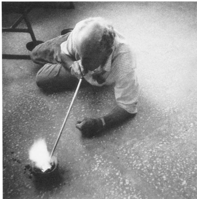
Fig. 1. Bryan Earl smelting tin in a crucible, July 1992, Celaller, Turkey. (Photo K.A. Yener)
