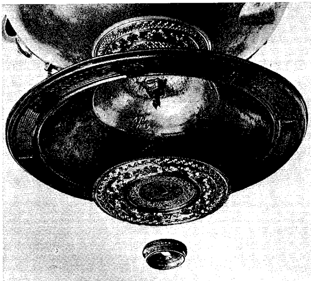
3. Exploded view of crystal mount, under-foot disc, and the end of the central bolt.
