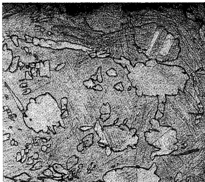
Fig 1. Microstructure at 500x of the massive transformation in 23% tin bronze gong sample collected by Professor Harold C. Conklin of Yale as part of his study of the Ifugao. See Goodway and Conklin, "Quenched High-tin bronzes in the Philippines," Archeomaterials 2, (1987) 1-27, for first publication of the occurrence of the massive transformation in tin bronze
