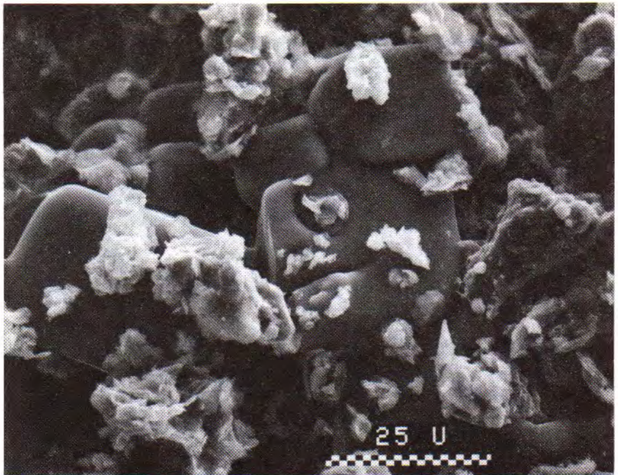
Figure 3 B. Detail of a group of sodium chloride crystals. Note the brick debris that has resulted from the fracturing produced by the growth of the crystals.
