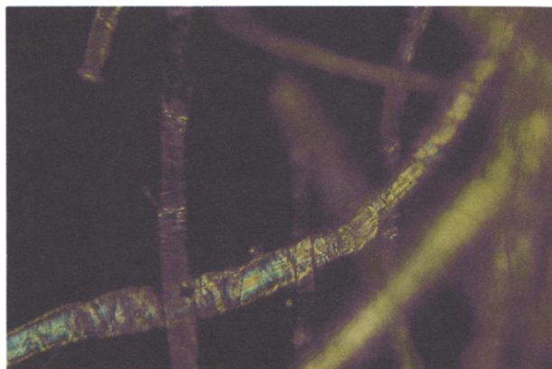
Plate 2: Red plate test of flax. Note the yellow color of the vertical fiber. 165x, 90° crossed polars, first order red compensator plate in 45° position.
