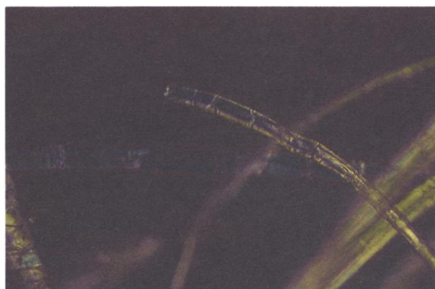
Plate 3: Red plate test of flax. Yellow fiber of Plate 2 rotated 90° to horizontal position. Note blue color. 500x, 90° crossed polars and red plate.
