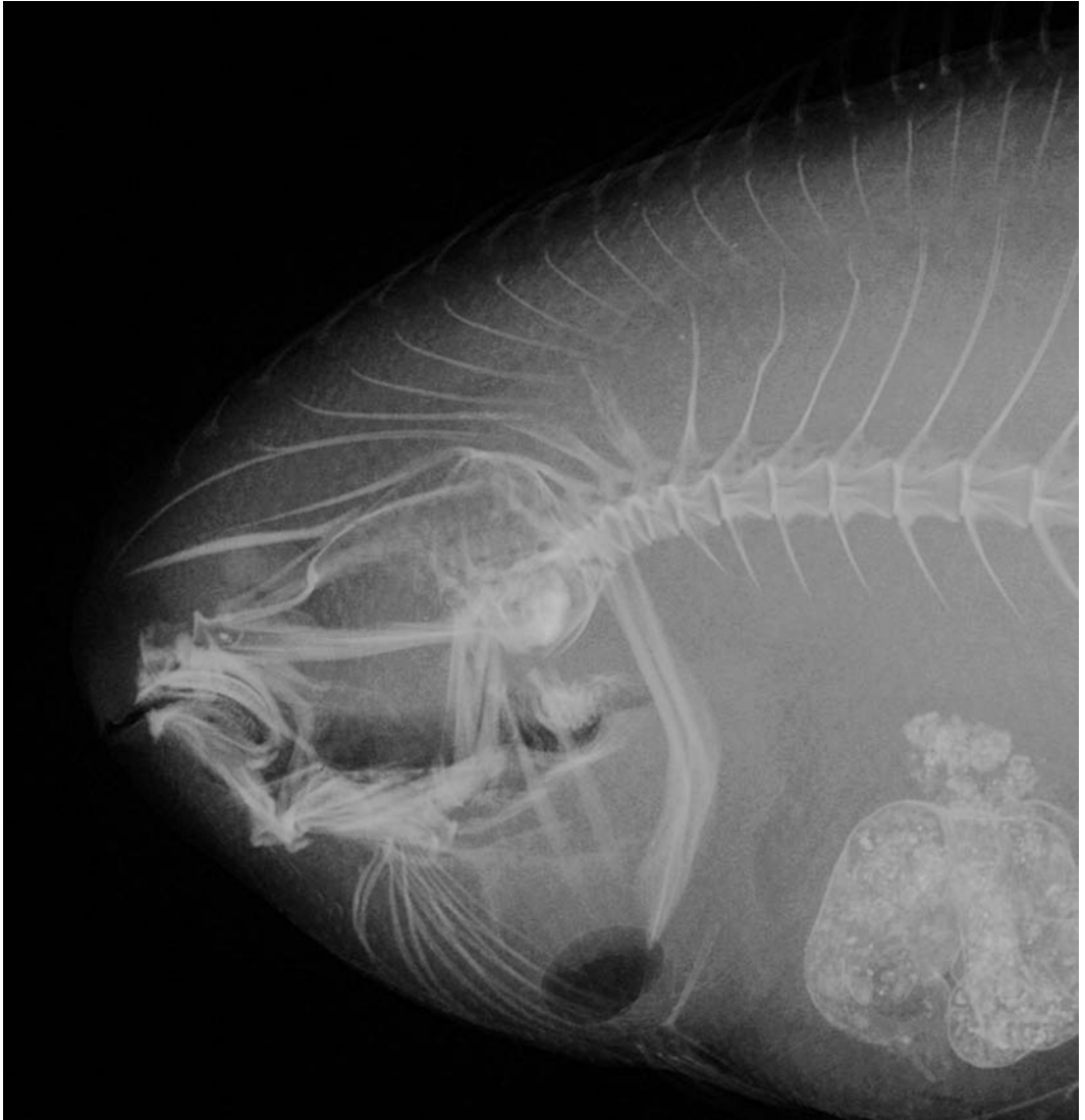
Fig. 3. Digital radiograph of anterior region of holotype (USNM 378272) of Symphurus ocellaris depicting the 1–3–4 pattern of interdigitation of anterior, dorsal-fin proximal pterygiophores and neural spines characteristic of this species. (See Munroe, 1992 for detailed information on ID patterns among symphurine tonguefishes)
