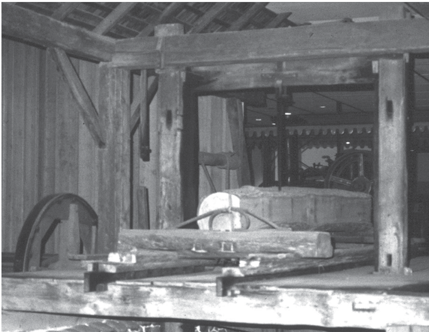
Figure 25 (left). The ratcheting function of the sled coordinated with the up and down action of the blade renders a perfectly regular set of chatter marks.
