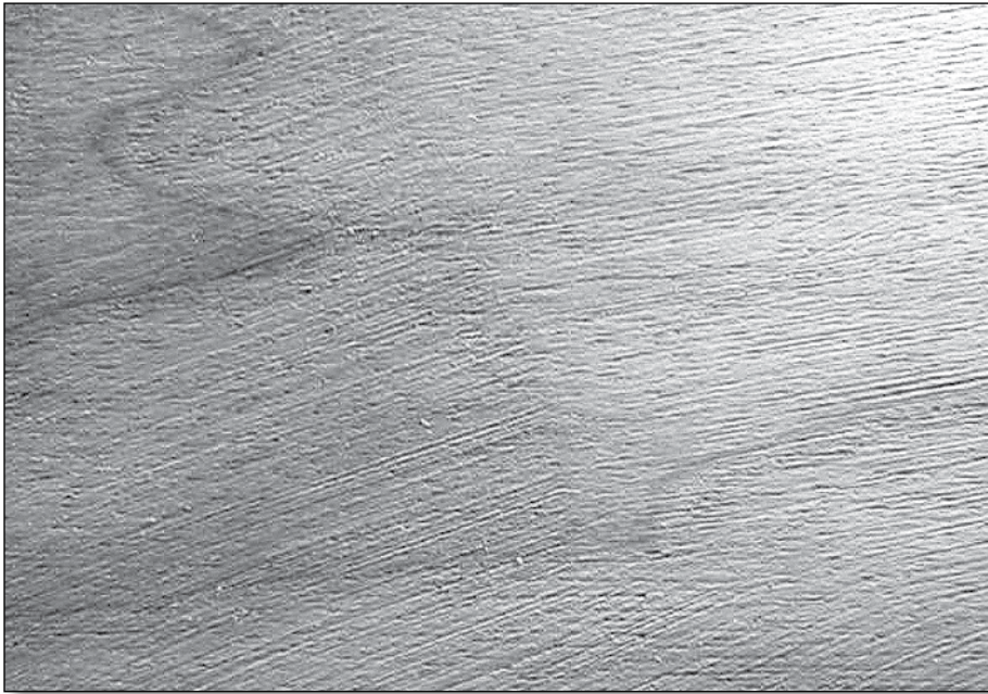
Figure 32 (above). Compared to the scraper, belt sanding leaves a coarser, abraded surface.
