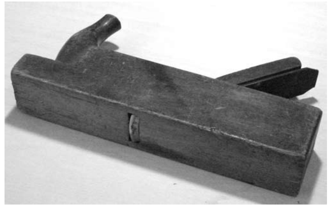
Figure 18 (below, bottom). A scrub plane renders a fairly flat, “guttered” surface reflecting the iron profile.
