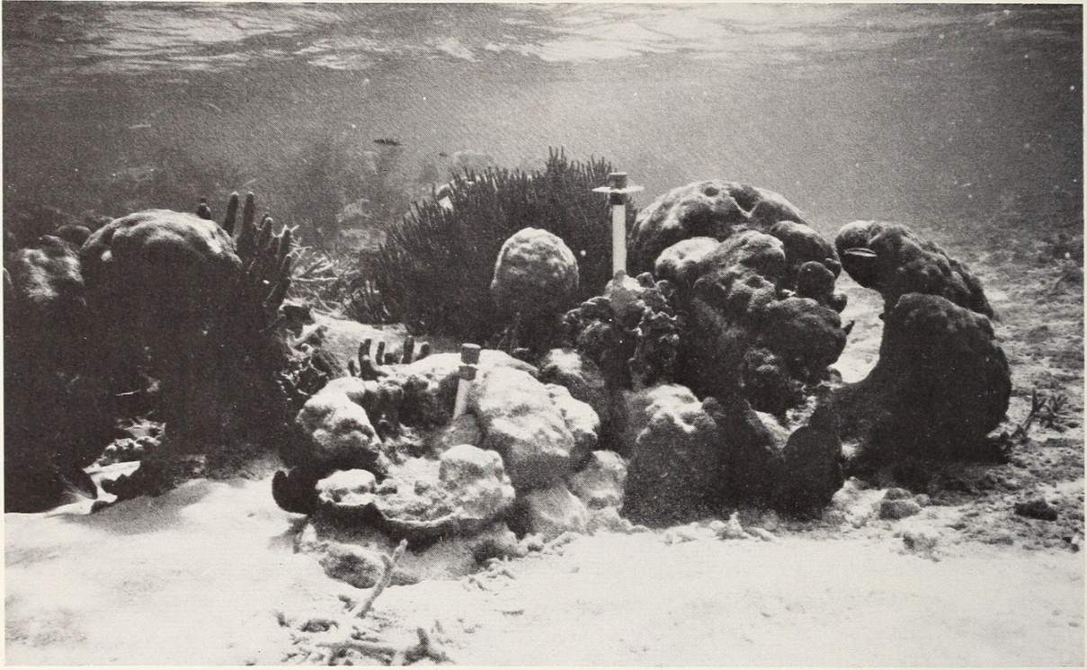
FIGURE 63.—Patch reef zone substrate station, Carrie Bow Cay, showing location of plates above the sediment-water interface.
