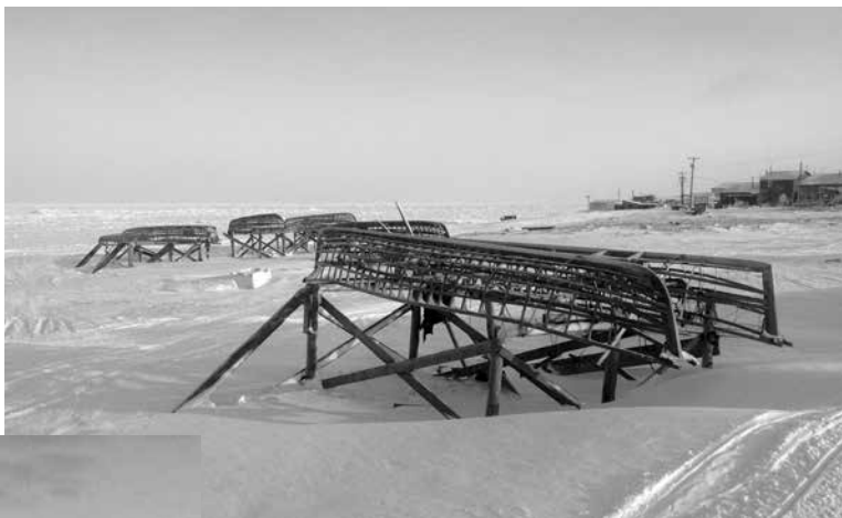
Left: A wooden boat frame with the remains of disintegrated skin cover on the beach in Gambell. October 2017
