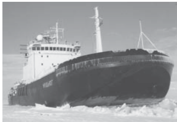
Thysen-Waas type hull form - a revolutionary hull design
