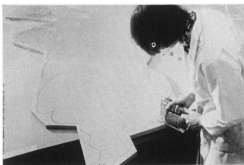
FIG. 9 Final cutting of cured complex curved panel.
