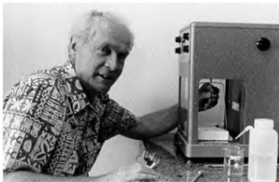
Richard Fiske uses a high-precision analytical balance to measure the specific gravity of a pumice sample taken from a Japanese volcano. He hopes to learn how deep in the ocean pumice can be formed and to be able to estimate the depth at which it can be erupted. (Don Hurlbert photo)
