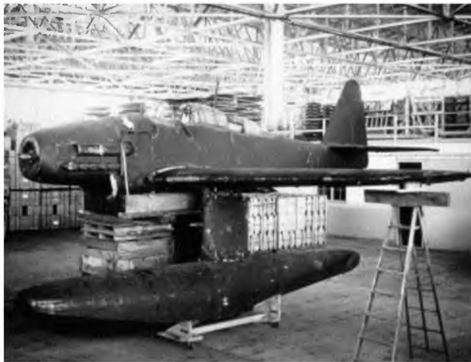
This photograph shows the Aichi M6A1 Seiran at Park Ridge, Ill., before it was transferred to the National Air and Space Museum's Garber Facility. The float attached to the bottom of the plane would allow a bomber returning from an attack to land on water near the mother ship.
