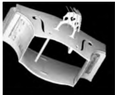
Using a CT scanner, researchers can study fragile objects, such as this rare 18th-century Stradivarius cello, in a noninvasive way.
