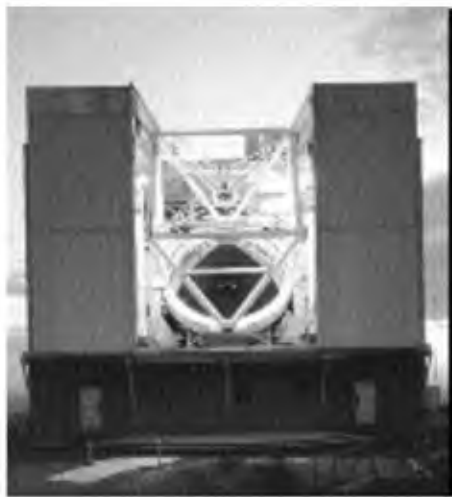
The Multiple Mirror Telescope now has just one mirror instead of six.
