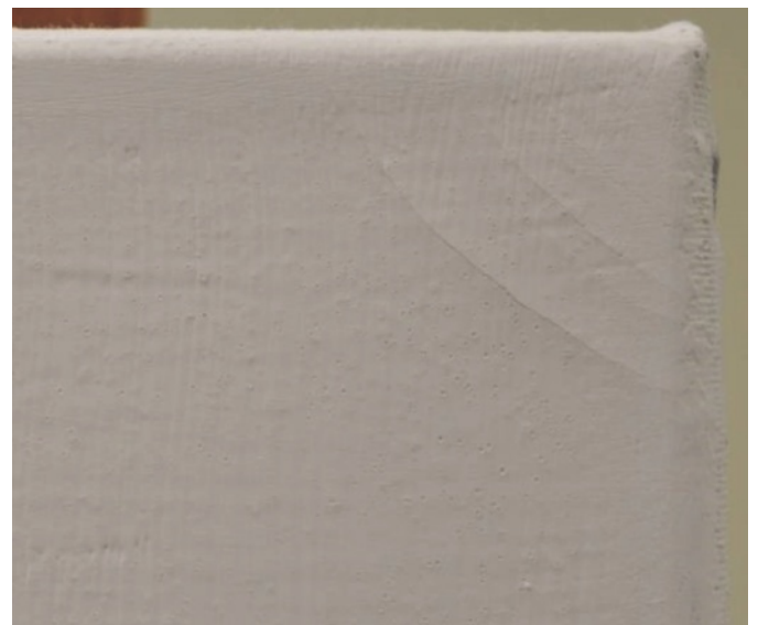
Figure 8. Sample 1. After 14 RH sets, corner AD had 5 cracks, 3 of which are fine and thus difficult to capture photographically, and 1 faint crack
