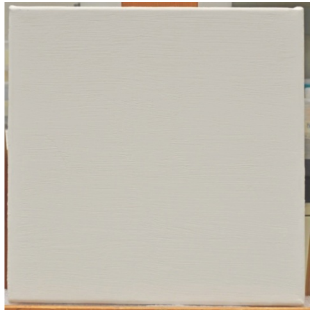
Figure 17. Sample 6, whole front. After 14 RH sets, no cracks developed
