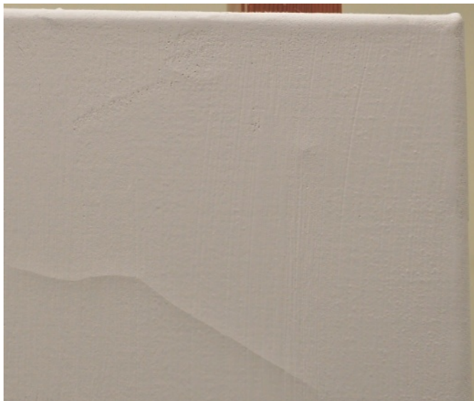
Figure 12. Sample 5, corner AD. After 14 RH sets there were no corner cracks, but there was a mechanical surface crack measuring ~10 cm and located ~11 cm from the right edge
