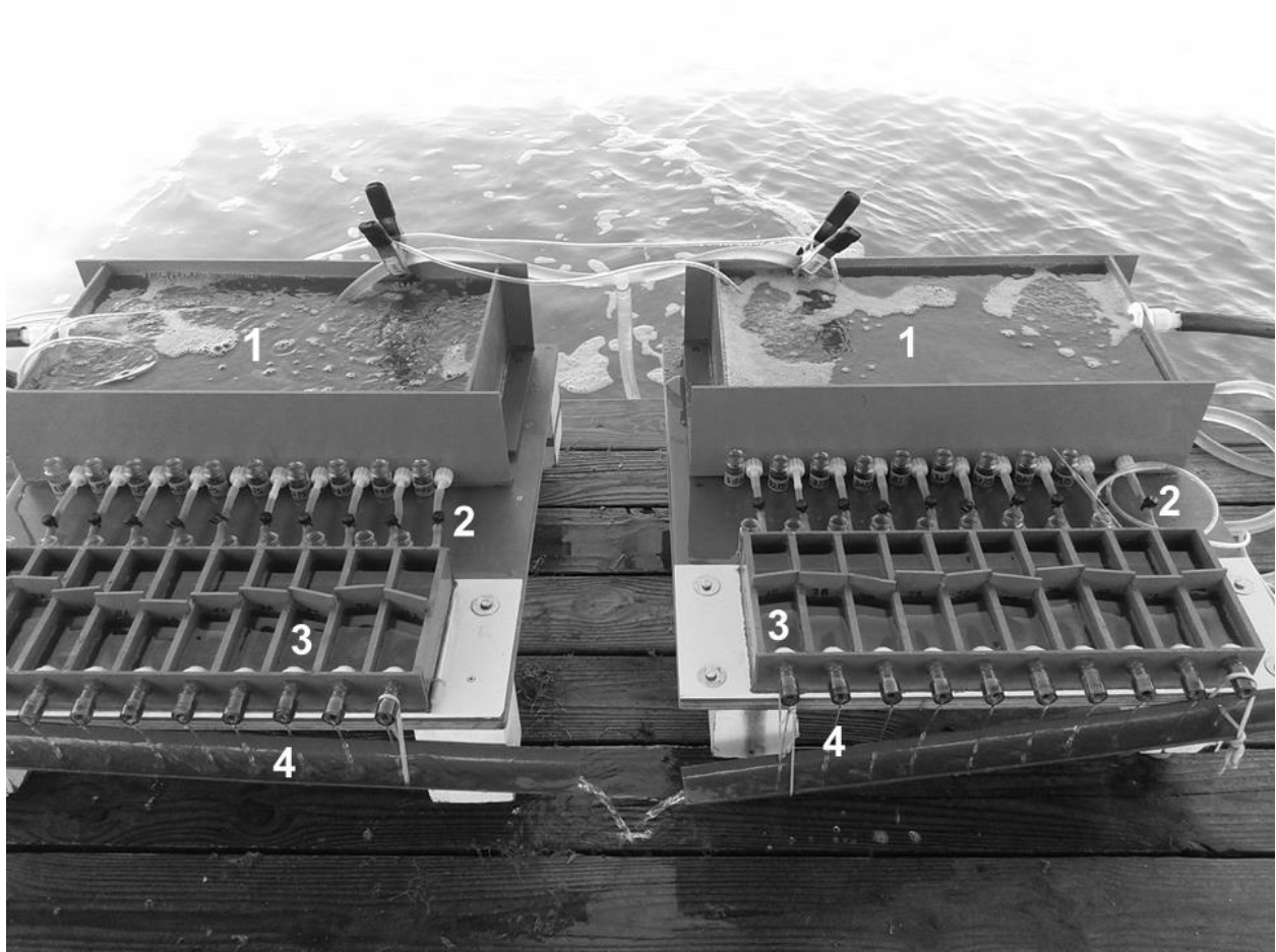
355 Fig. 1: Image of the two portable, flow-through devices used for the filter feeding experiments. 1: PVC 356 “reservoir” tank; 2: plastic tubes with valves to regulate flow connecting the “reservoir” tank with each 357 individual chamber; 3: individual chambers that each hold a single bivalve; 4: overflow of the chamber. 358
