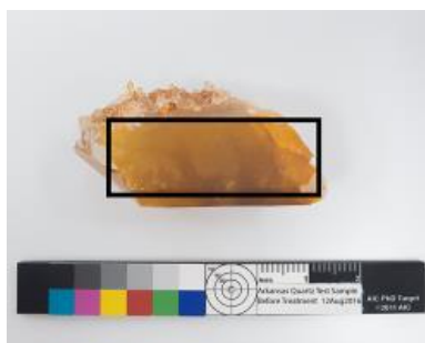
Fig. 1. Growth face of Arkansas quartz used for test cleaning, prior to treatment; region of interest is outlined in black rectangle-
