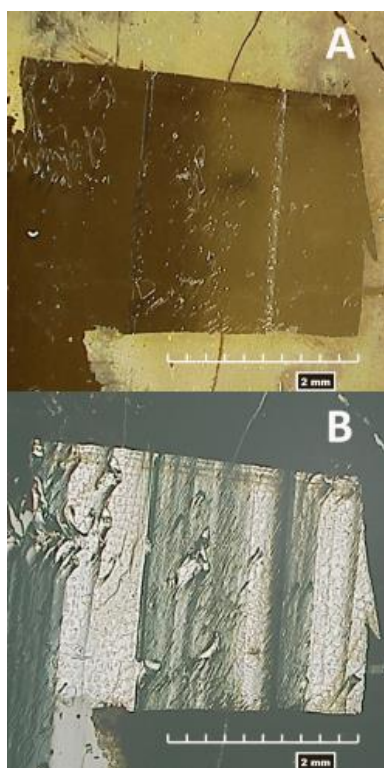
Fig. 5. (A) Spot 1 ( F=2.65 \text{ J/cm}^2 ) appears clean with ring lighting and (B) Spot 1 under coaxial lighting conditions reveals surface patterning of thin-film residue-
