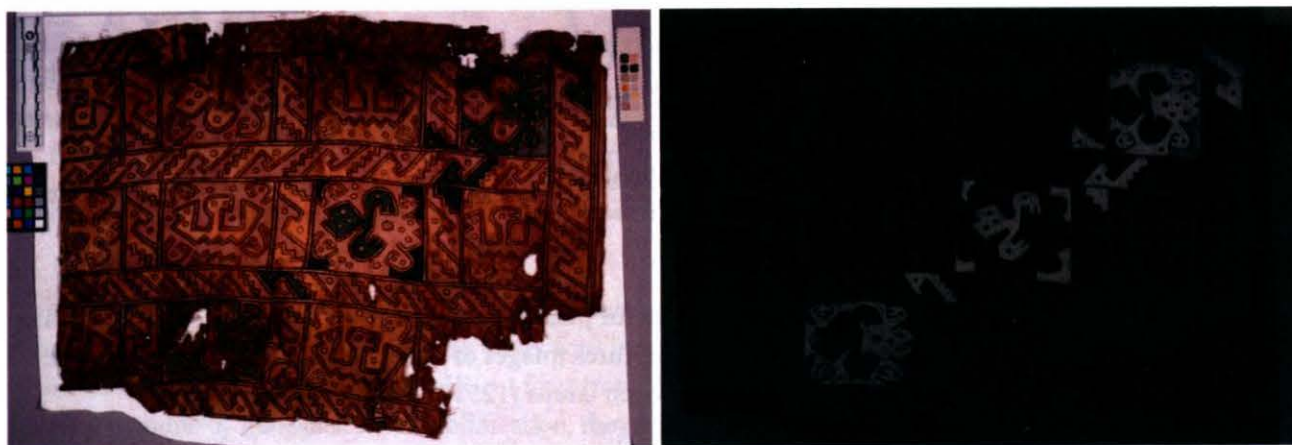
Figure 5: NMAI 23/9038 visible light image (left) and image subtraction of the 735 nm bandpass image and the 660 nm bandpass image emphasizing the areas of indigo in resulting image (right)
