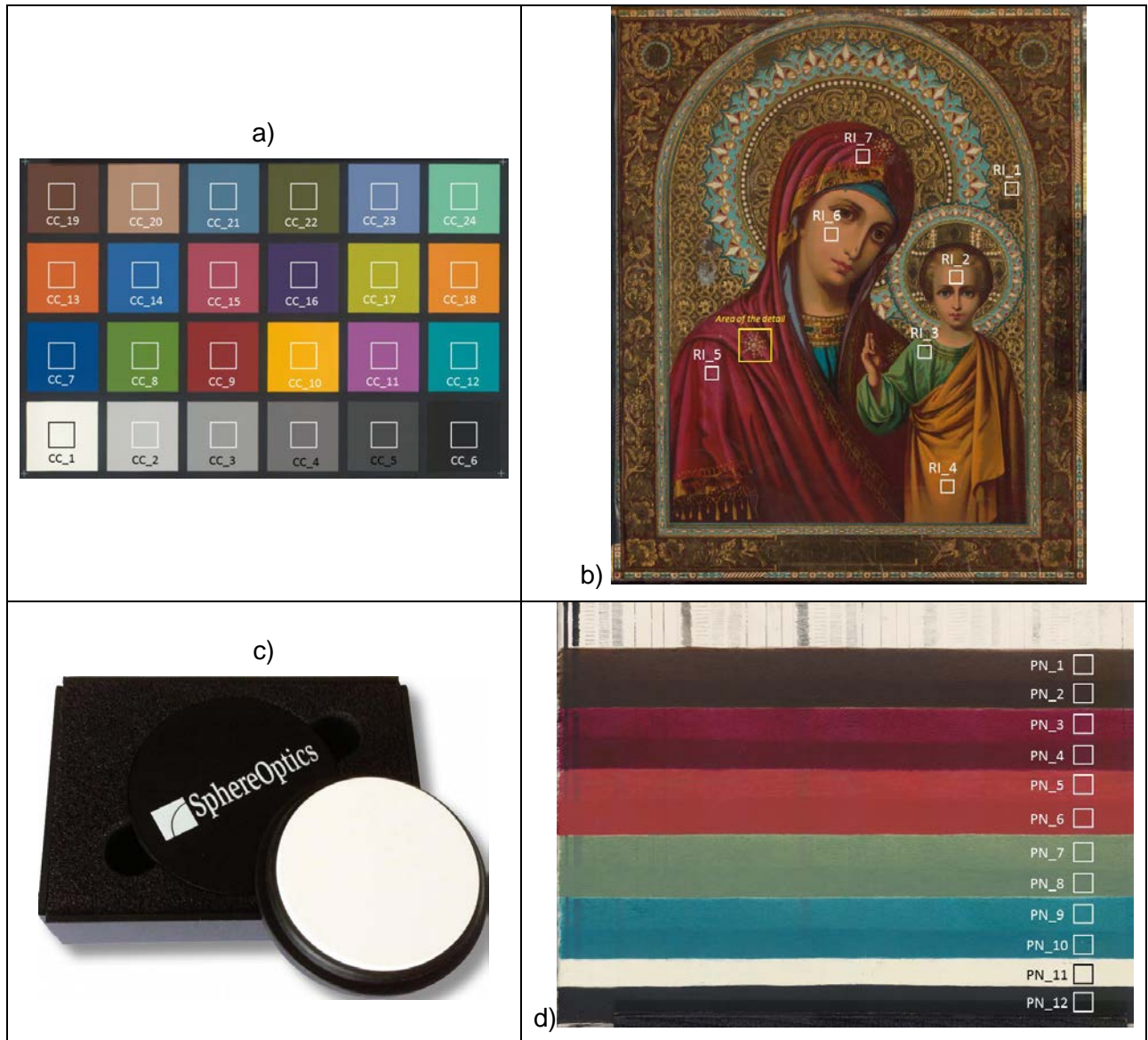
Figure 1: a) X-Rite ColorChecker with sampling areas for colorimetric and spectral analysis. b) Russian icon with sampling areas for colorimetric and spectral analysis. c) SphereOptics Zenith Polymer Wavelength Standard. d) Replica panel painting with sampling areas for colorimetric and spectral analysis.
