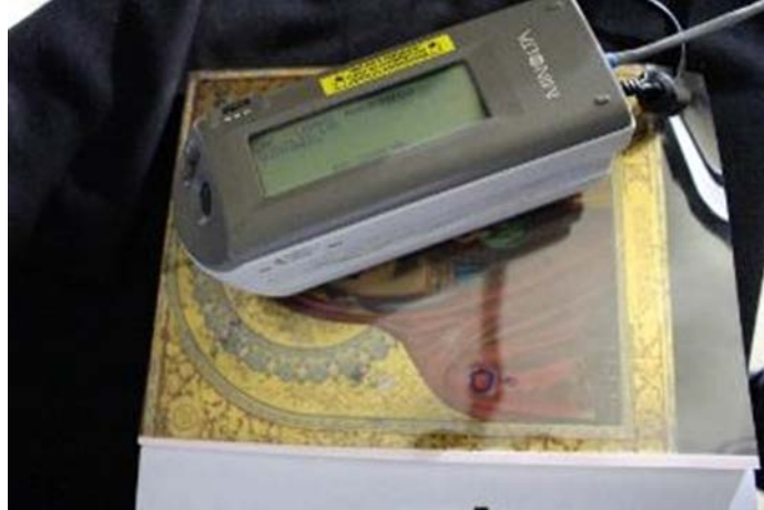
Figure 3: Minolta CM-2600d measuring reflectance spectra on selected areas of the Russian icon.
