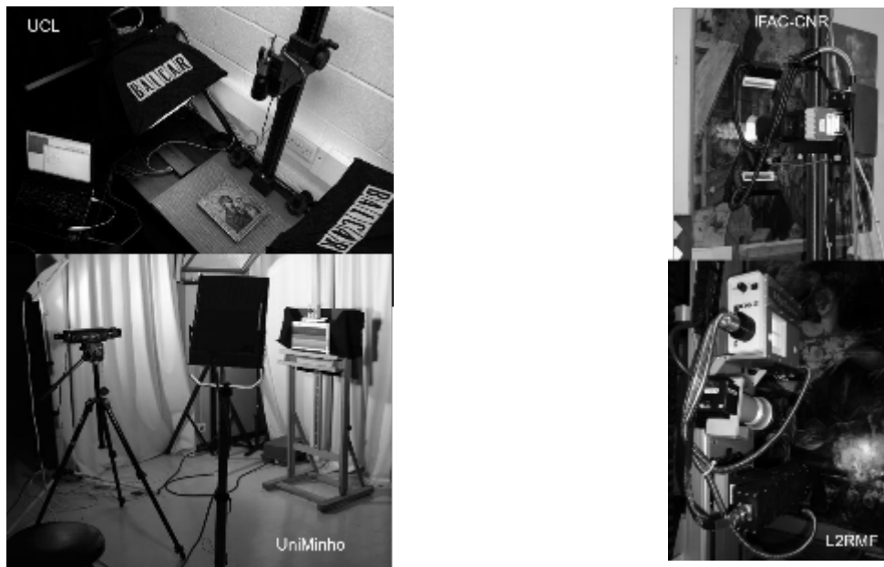
Figure 2: Different spectral imaging devices used within RRT. Left MSI; right HSI.
