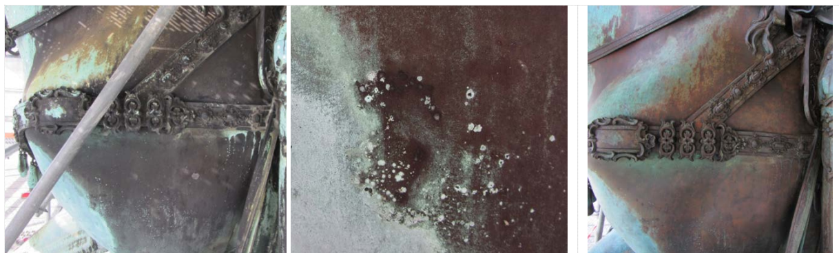
Figure 6. Aspects of a transition zone between the black and green patinas (left). The small bright dots of nantokite identified in the detail (center) show that they are in fact pustules protruding through the black cover thus acting as an entrance window of the corrosion agents to the underneath copper alloy. The same area after cleaning (right).
