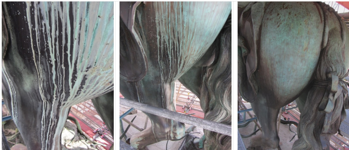
Figure 7. Aspect of a zone with highly a contrasting colored pattern before (left), after cleaning (center) and after cleaning and artificial patination (right).
