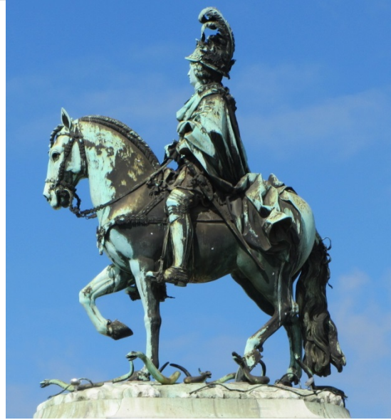
Figure 1. D. José I statue in Lisbon. East view (left) shows the prevalence of dark patinas, while in the west side (right), more exposed to the marine winds and rains, green patinas prevail.
