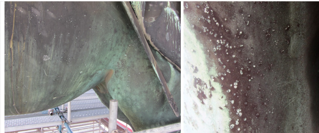
Figure 4. Aspect of the green patina covered with a blackish layer (left), and a detail of the surface pustules and disruptions (right).
