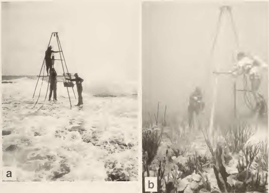
Figure 6. Working with hydraulic-operated coring equipment: (a) Above water drilling the Holandés Ridge, Panamá. 1993. (b) At a depth of 15 meters, coring a relict reef off the southeast coast of St. Croix. 1976.
