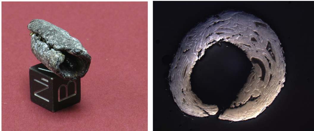
Fig. 8. Meteoritic metal bead formed from the Anoka iron using wood-fueled fire for heating and lithics for deformation. Right: Cylindrical bead formed by rolling a flattened sheet. Scale cube is 1 cm on a side. Left: Reflected light photomicrograph of a cross section of the bead illustrating the deformation of the Widmanstatten pattern. Bead is 1 cm in exterior diameter.
