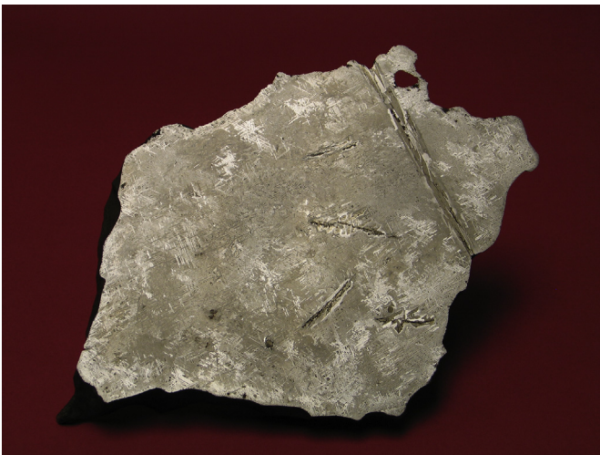
Fig. 7. Slice of the Anoka iron exhibiting prominent schreibersite, including a 0.5 × 12 cm skeletal crystal that bisects the slice, and a fine Widmanstatten pattern. Maximum dimension of the slice is 26 cm.
