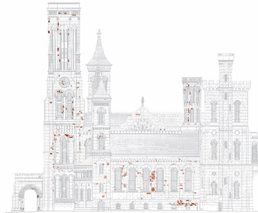
Figure 10: West elevation of the Castle modified from the Smithsonian's 2002 Master Plan Survey. Varnish patches are highlighted in red.
