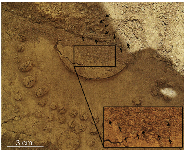
Fig. 14. The soil Portage as imaged by MAHLI and investigated by APXS (both on sol 89). Note the high-fidelity casting of the APXS contact plate (including the larger screw hole on the very bottom). Arrows mark some of the coarse grains within the field of view of the APXS, which was about 3.1 cm in diameter at a standoff distance of 2 cm. Image ID: Background image: Detail of 0089MH0120001001E1. Top insets: 0089MR062800000E1 and 0089MR062900000E1. Bottom inset: Detail of 0089MH0122001001E1.
