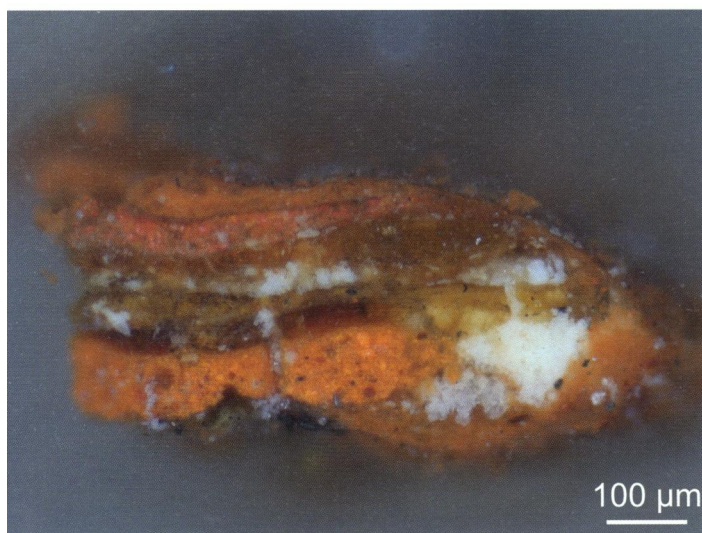
Fig. 5. Cross section of fig. 1 from an area of red background behind the Virgin's robe, dark-field visible-light image. Challacolloite salts can be seen as white clusters growing in between surface decoration layers.
