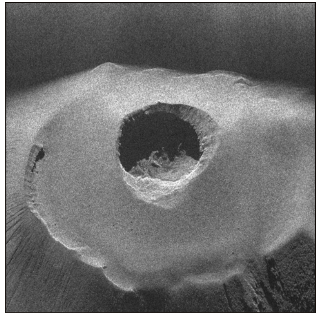
Figure 8. Radar image of Asama's summit crater taken from a Cessna on 15 December 2004 by the Geographical Survey Institute, Japan. N is up. Radiated microwaves were transmitted from the N, 2 km from the crater, with the off-nadir angle of 55 degrees. Courtesy of Geographical Survey Institute.
