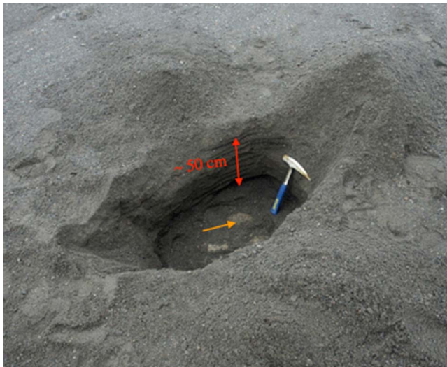
Figure 8. A trench dug into sediments (see Figure 6b for location) overlying the December 1974 flow (indicated by the orange arrow) provides evidence that there has been \sim 10 later storm events in the Ka‘ū Desert capable of generating runoff and flow through the drainage networks developed in the Keanakāko‘i tephra. Each flow event is represented by a flood couplet \sim 5 cm thick that comprises a coarser- and finer-grained layer. An analysis of state climatic records indicates that the storms with the highest precipitation typically occur during the winter months when southerly winds create prolonged stationary disturbances, generating so-called “kona storms.”
