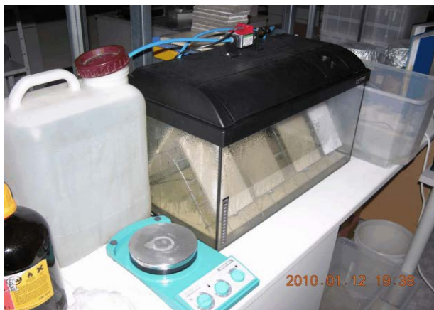
Figure 5. Principle of the dynamic CSTB-Test: (left) Inoculation solution with algae; (center) Moist incubation chamber with illuminated samples in front; (right) Collector for sprayed algal solution.
