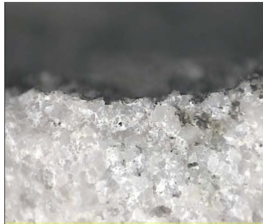
Figure 4. Detail of the previous figure showing that the microbial biofilm rarely reaches deep into the stone profile.
