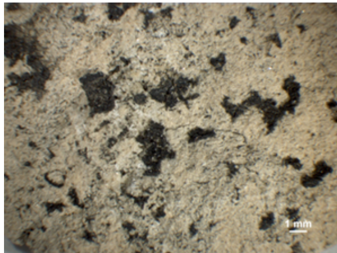
Figure 14. Stereomicroscope view of the sample surface (#7) with localized biocolonization.
