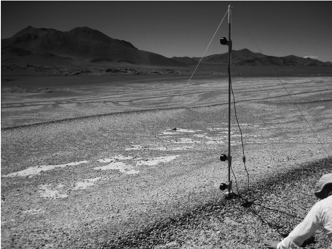
Fig. 3. Tower on crest of a megaripple at the Purulla site. Wind was blowing perpendicular to the megaripple crest. A non-logarithmic wind profile was observed at this location, possibly related to the Bernoulli effect of compressed flow lines moving up the stoss side of the bedform. JRZ photo, 12/6/10.
