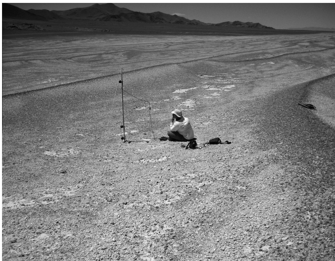
Fig. 1. Wind profile equipment in a trough between megaripples at the Purulla site, looking north. Subsequent measurements were obtained at locations across the megaripple to the right of the tower. JRZ photo, 12/6/10.
