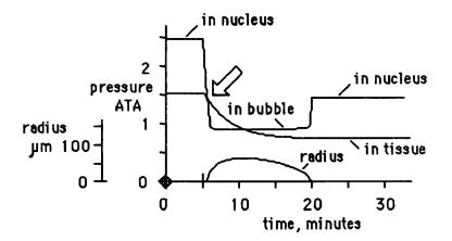
Fig. 5. In a nucleus slightly larger than the one of Fig. 4, a crossover allowed transformation into a bubble.
