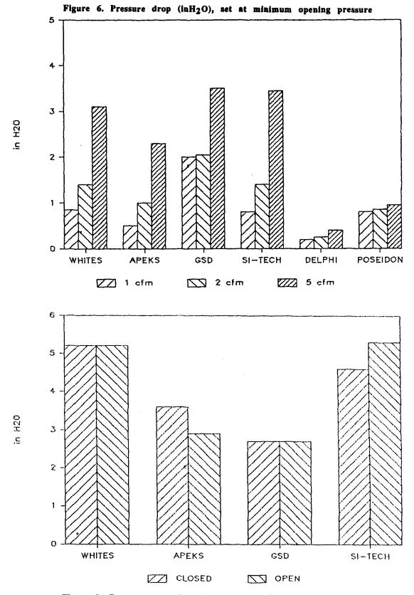
Figure 7. Pressure drop (inH2O), 5 cfm min/max opening pressure
