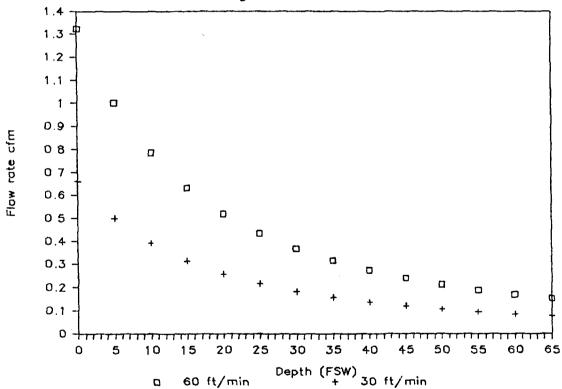
With a higher starting volume, figure 2 shows the flow rate requirements placed on the exhaust valve if the starting volume is twice as large as that in fig.1 (0.5 cu ft.). As one would expect, the flow requirement is also twice that of lower starting volumes.
