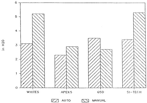
Figure 8. Pressure drop (inH<sub>2</sub>O), 5 cfm auto and manual operation
