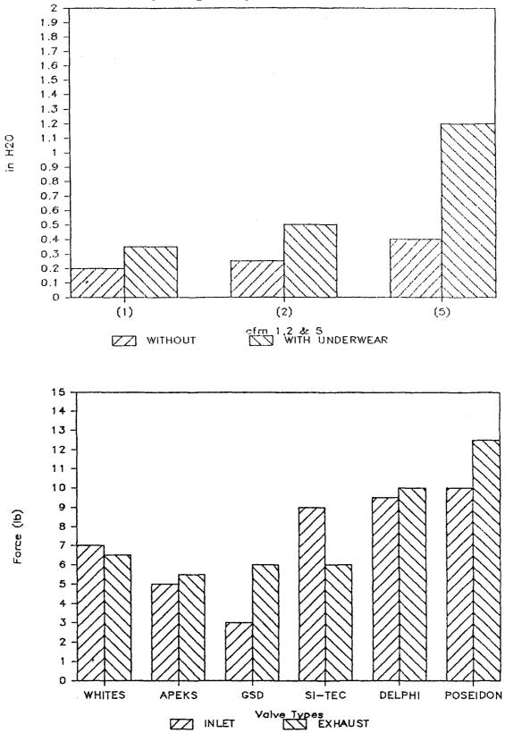
Figure 10. Pressure drop (in H2O), Delphi valve with and w/o underwear behind valve
