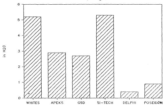
Figure 9. Pressure drop (inH2O), 5 cfm
