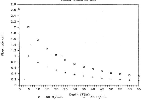
Figure 2. Exhaust valve flow rate requirements Starting volume: 0.5 cu.ft.
