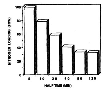
Figure 3. U.S. Navy theoretically allowable nitrogen loading
