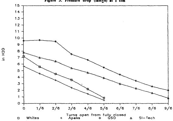
Figure 3. Pressure drop (inH<sub>2</sub>0) at 1 cfm
