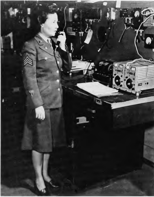
FIGURE 16.—Sergeant Lois Herring, WAC, bench-tests an aircraft radio set, prior to its actual installation in an airplane. Sgt. Herring frequently went on cross-country flights as a radio operator. (NASM/USAF neg. A-33930A.C.)
