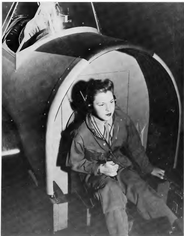
FIGURE 13 (above).—Women's Army Corps officer is shown instructing a student in a Link trainer. (NASM/USAF neg. 27503A.C.)
