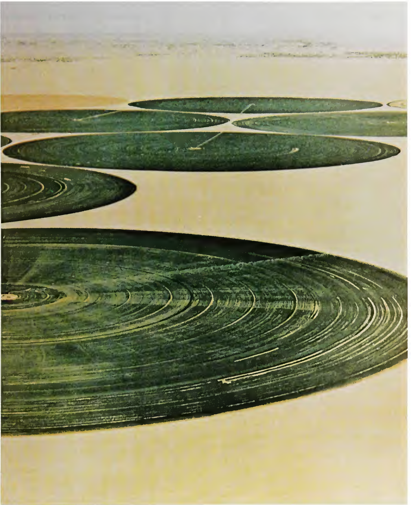
FIGURE 80.—Photograph of Kufra area showing the circular patterns caused by huge rotating sprinklers 560 m in radius. (Photo courtesy of Derek Bayes, Aspect Picture Library Ltd, Surrey, England)
