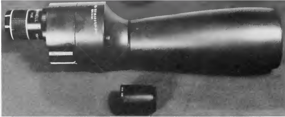
FIGURE 37.—The 20-power enlarging telescope used by the ASTP crew to spot small observation targets. (Courtesy of J. A. Taylor)
