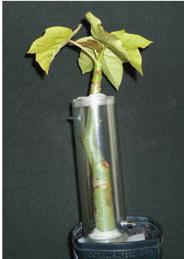
Fig. 1. Mature stem of Jatropha curcas enclosed by a cylindrical gas-exchange cuvette (17 × 5 cm inner dimensions). The young foliated stem-tip is outside the cuvette. The air inlet is at the bottom, the air outlet at the top.
