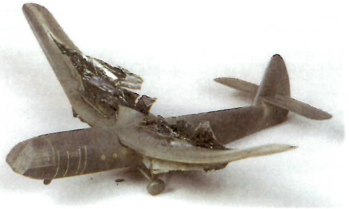
A model of a British Airspeed Horsa. Models like this were used to teach aircraft recognition during World War II. Seven decades later, many of these early examples of injection-molded cellulose acetate plastic are disintegrating spontaneously in the National Air and Space Museum collection. Photo: E. Keats Webb, Museum Conservation Institute, Smithsonian Institution.
