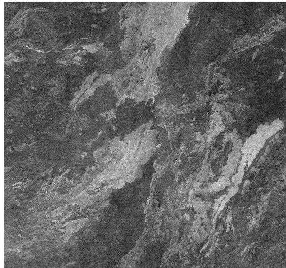
Figure 9. Magellan 12.6 cm radar image of lava flows north of Didilia Corona (approximate image center 19.6°N, 40.5°E). Image width 180 km and resolution 150 m per pixel. Note the rough-surfaced, radar-bright flows with central channels extending downhill from lower left of image. The bright flow at center has been bisected by later smooth (radar-dark) lava flows, which have also flooded the channels.
