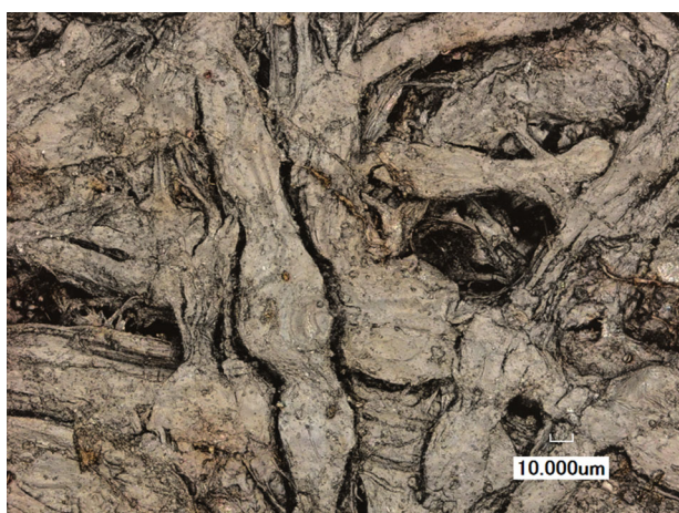
Fig 10. Reverse of stain A shows smooth surface of paper fibers with minimal fungal growth. Lesser amount of fungal deposits was consistent on all stains, throughout the entire reverse side of the paper sheet. Keyence VK9700 at magnification 1000x, scale bar: 10 \mu\text{m} .
