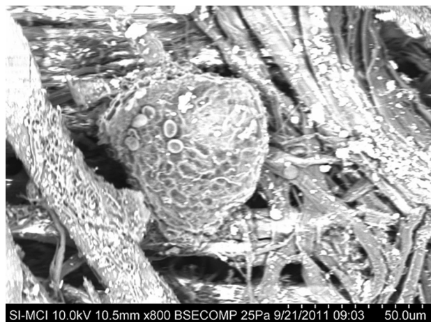
Fig 8. Stain B. SEM-VP micrograph of the pigmented fruiting body anchored to paper fibers. Paper fibers are used as a physical support for the fruiting structure. SEM-VP Hitachi S 3700N, magnification 800x, BSE, pressure 40.Pa, power of electron beam 10.0kV, scale bar, 50 \mu\text{m} .
