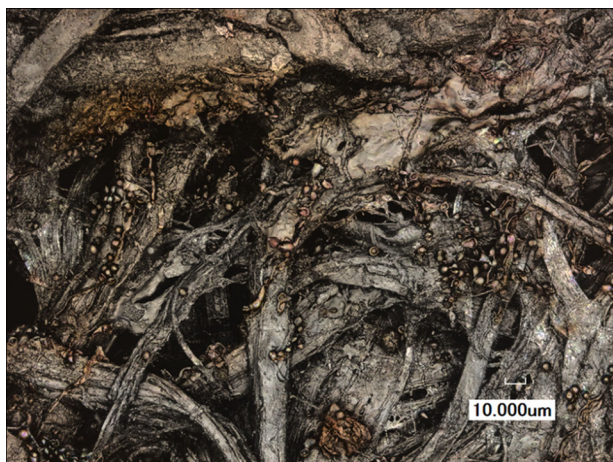
Fig 9. Stain A. Surface morphology of paper with fungal cells captured with 3D confocal laser scanning microscope (CLSM). Laser scanning over fungal cells in xyz direction produced 3D image with accurate height of the cells and paper fibers. Distribution of semi-spherical cells is visualized with orange color on the background of brown fibers. Lighter coloration of cells is due to their elevated position on the surface of fibers. Keyence VX9700 series at magnification 1000x, scale bar: 10 \mu\text{m} .
