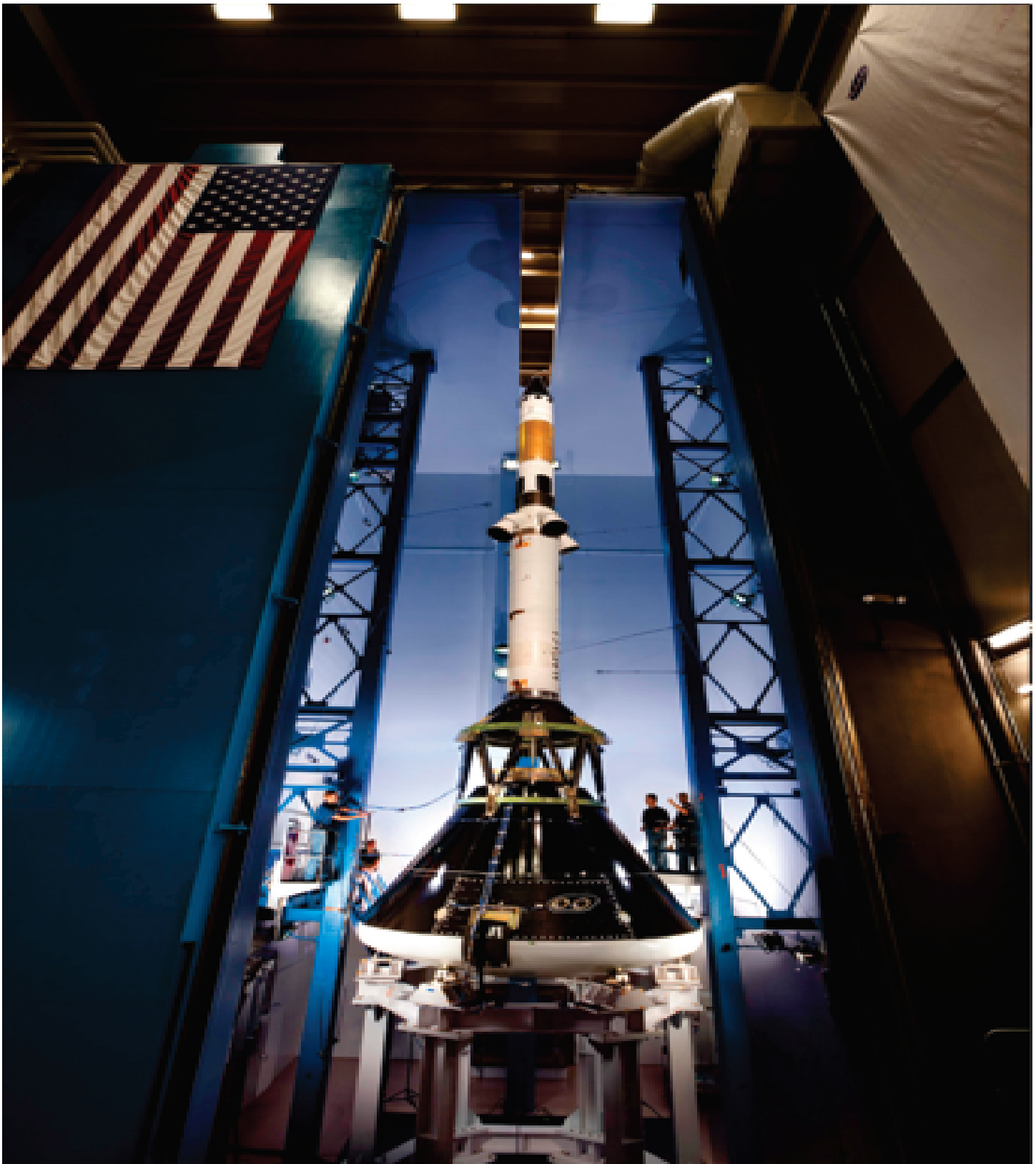
Technicians position microphones around the Orion MPCV and LAS test articles in preparation for the second round of testing in the acoustic chamber at Lockheed Martin's facilities near Denver on August 17, 2011. The vehicle was bombarded by acoustic levels of 150 decibels to simulate conditions during launch and abort if necessary. (Source: Lockheed Martin)
