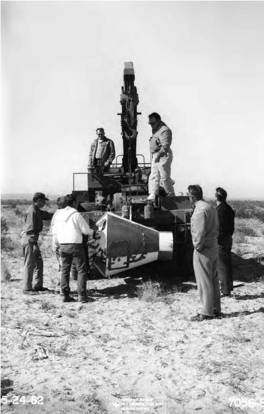
NASA engineers recovering the Gemini paraglider after a test in the Mojave Desert. NASA.
