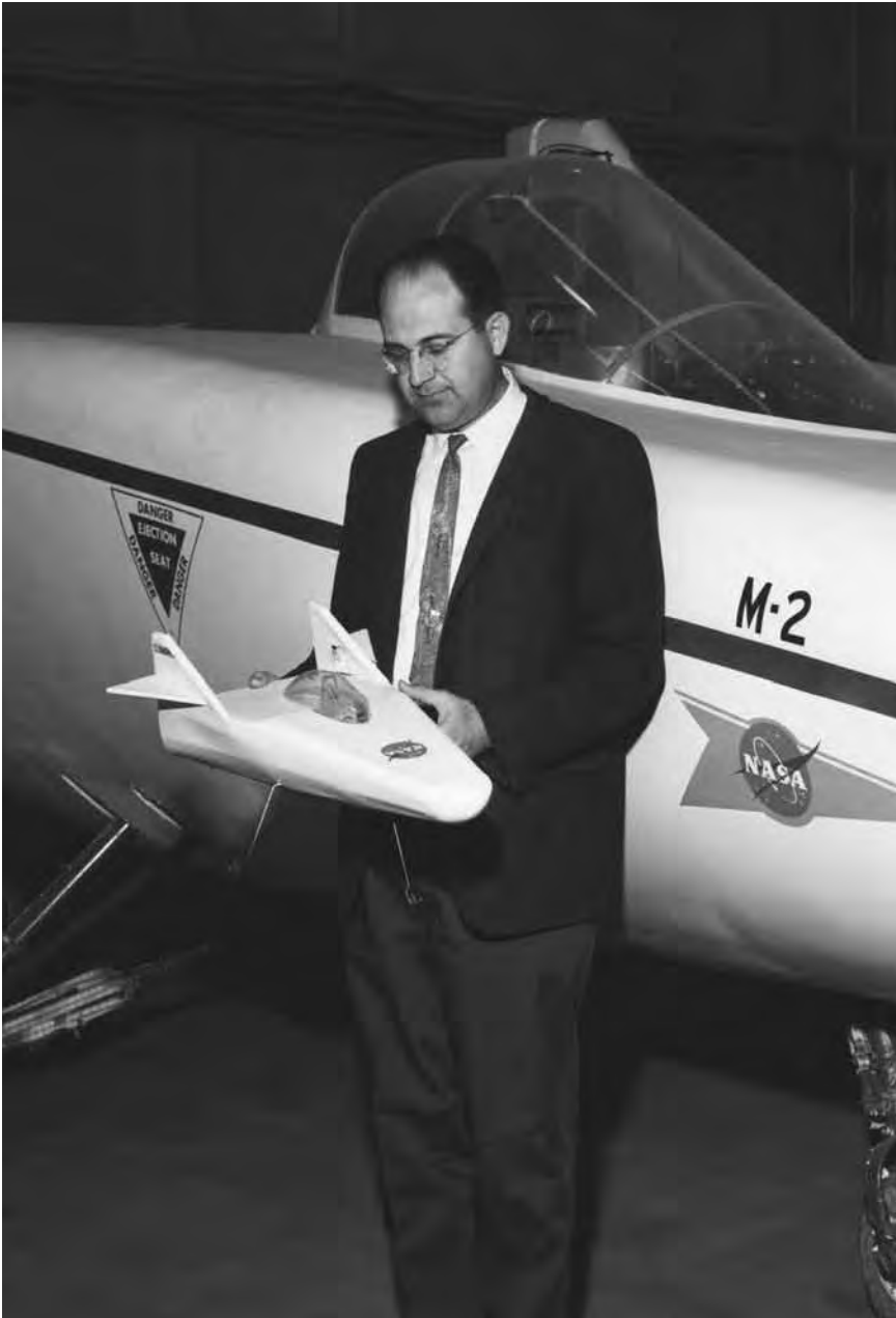
NASA engineer Dale Reed holds a model of the M2-F1 lifting body with the full-scale version directly behind him in 1967. In support of the M2 lifting body program in the early 1960s, Reed had built a number of small lifting body shapes and drop-tested them from a radio-controlled mothership. NASA E-16475.
