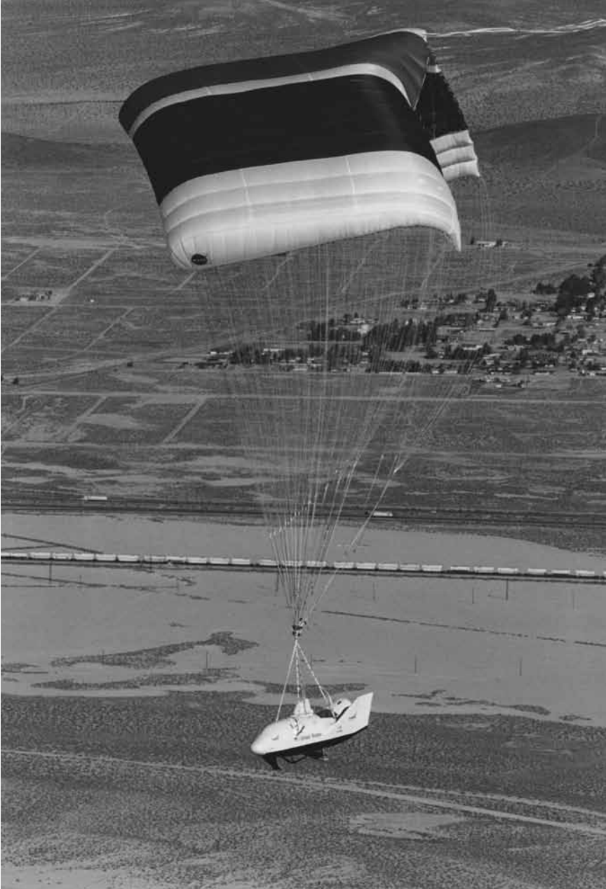
An X-38 test vehicle glides down under a giant parafoil toward a landing on Rogers Dry Lake near NASA's Dryden Flight Research Center during its first free flight on November 2, 2000. The huge 7,500-square-foot parafoil enabled the vehicle to land in an area the length of a football field. NASA EC00-0317-41.
