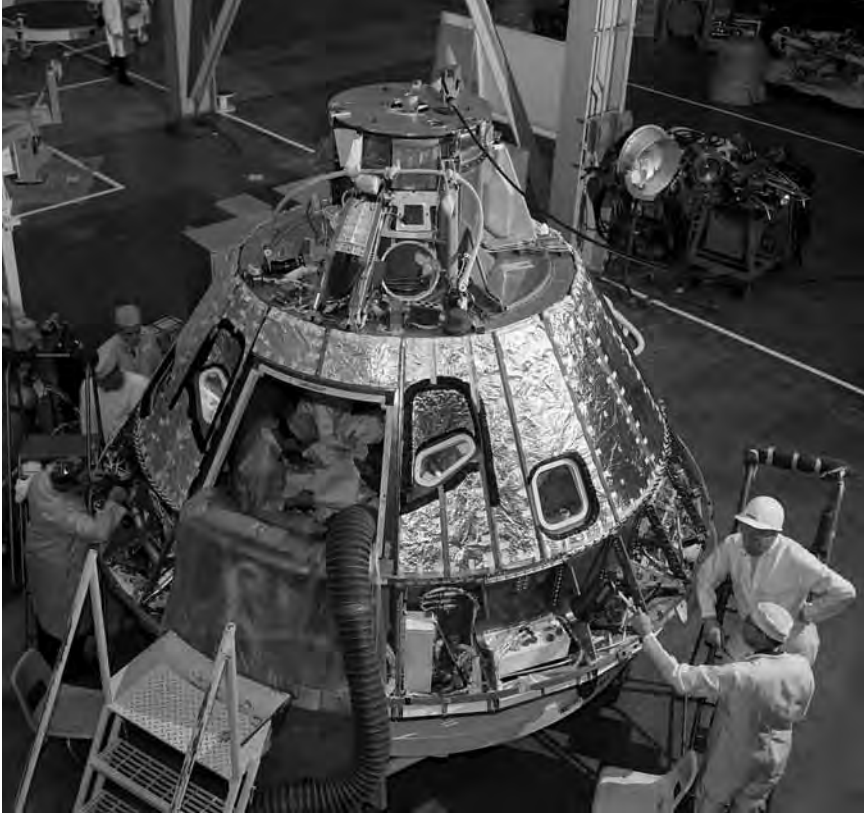
High-angle view of Command Module 012, looking toward the -Z axis, during preparation for installation of the crew compartment heat shield—showing technicians working on aft bay. This was the ill-fated Apollo 1 spacecraft. NASA s66-41851.
