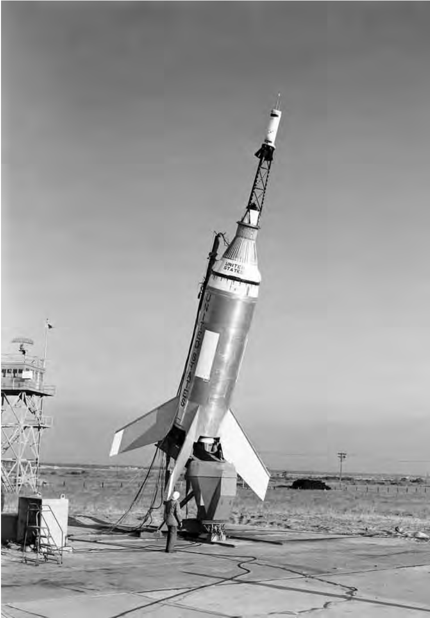
Little Joe 1 (LJ-1) was launched on October 4, 1959, at Wallops Island, VA. This was the first attempt to launch an instrumented capsule with a Little Joe booster. Only the LJ-1A and the LJ-6 used the space metal/chevron plates as heat reflector shields, as they kept shattering. Little Joe was used to test various components of the Mercury spacecraft, such as the emergency escape rockets. NASA L-1960-00104.
