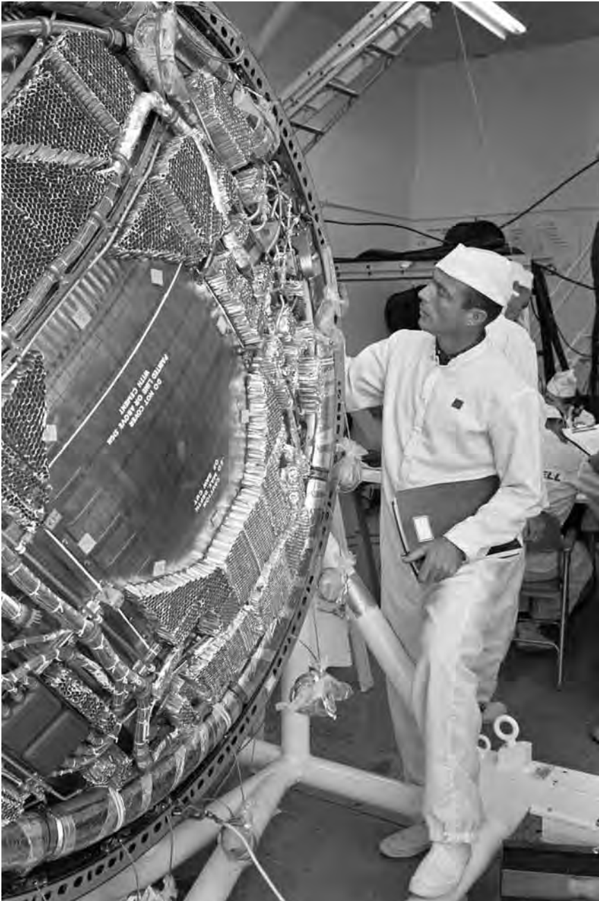
Inside Hangar S at Cape Canaveral, Mercury astronaut M. Scott Carpenter examines the honeycomb protective material on the main pressure bulkhead (heat shield) of his Mercury capsule, nicknamed "Aurora 7." NASA S62-01420.
