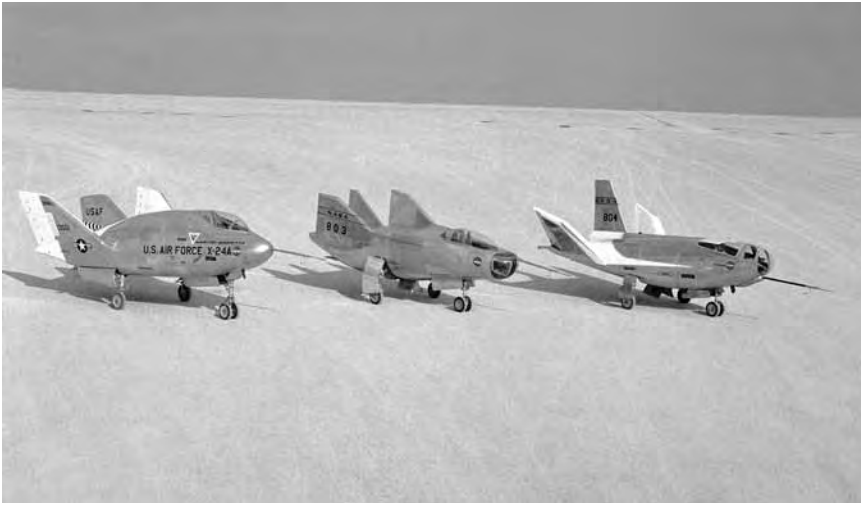
Three lifting body vehicles at NASA's Flight Research Center in California in 1969. Left to right: the X-24A, M2-F3, and HL-10. These aircraft helped pave the way for later spaceplane concepts. NASA EC69-2358.
