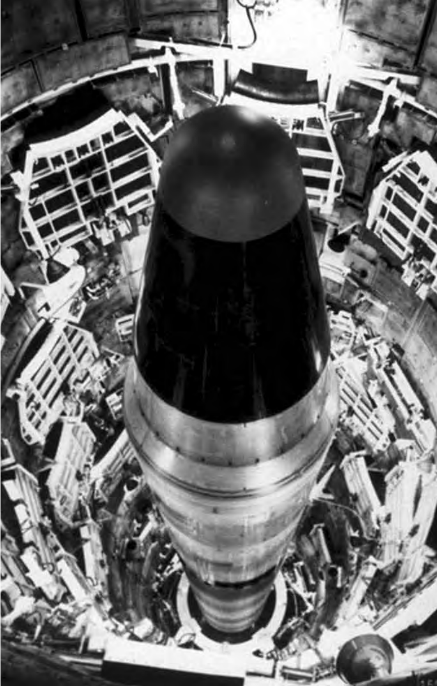
A Titan II intercontinental ballistic missile with an Mk 6 reentry vehicle. USAF.
