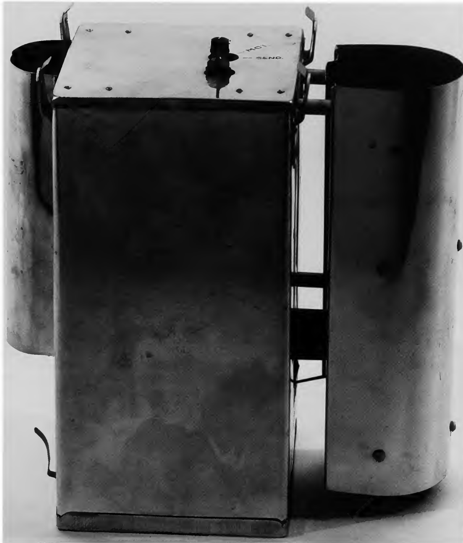
FIGURE 56.—A Gaw coding sonde, as redesigned by H. Hinzpeter in 1950. The mechanical parts and transmitter are enclosed in foil-coated, fiberboard box about 10×10×20 cm. Metal shields for the hair hygrometer and the bimetallic thermometer are on the left and right sides of the central box, respectively. In addition to their complexity and relatively high cost, the design principles of coding sondes made necessary the employment of sensors whose output was a mechanical displacement. This precluded any simple incorporation of improved sensors, whose output was a change in some electrical characteristic that were developed in the 1930s. (Instrument in NMAH collection, catalog number MHT 324241; Smithsonian photo 61906-C.)
