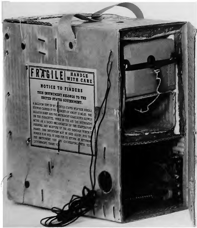
FIGURE 58.—A U.S. Weather Bureau radiosonde (left), circa 1942, based upon a NBS-Navy design, is housed in a foil-covered cardboard case, 22×11×22 cm. Two flaps open to reveal an electrolytic thermometer and a cylindrical array of hairs that operated a variable resistor. The hygrometer is mounted on white plastic molding and is enclosed in a semicylindrical white shield with louvers at the upper end. Batteries, a transmitter, and a “baroswitch” occupy the remainder of the carton. A similar sonde is shown (below) with the case cut away to allow most of the components to be seen. (Both instruments in NMAH collection, catalog number MHT 312798, above; catalog number MHT 322315, below; Smithsonian photos 61905-B and 61905, respectively.)
