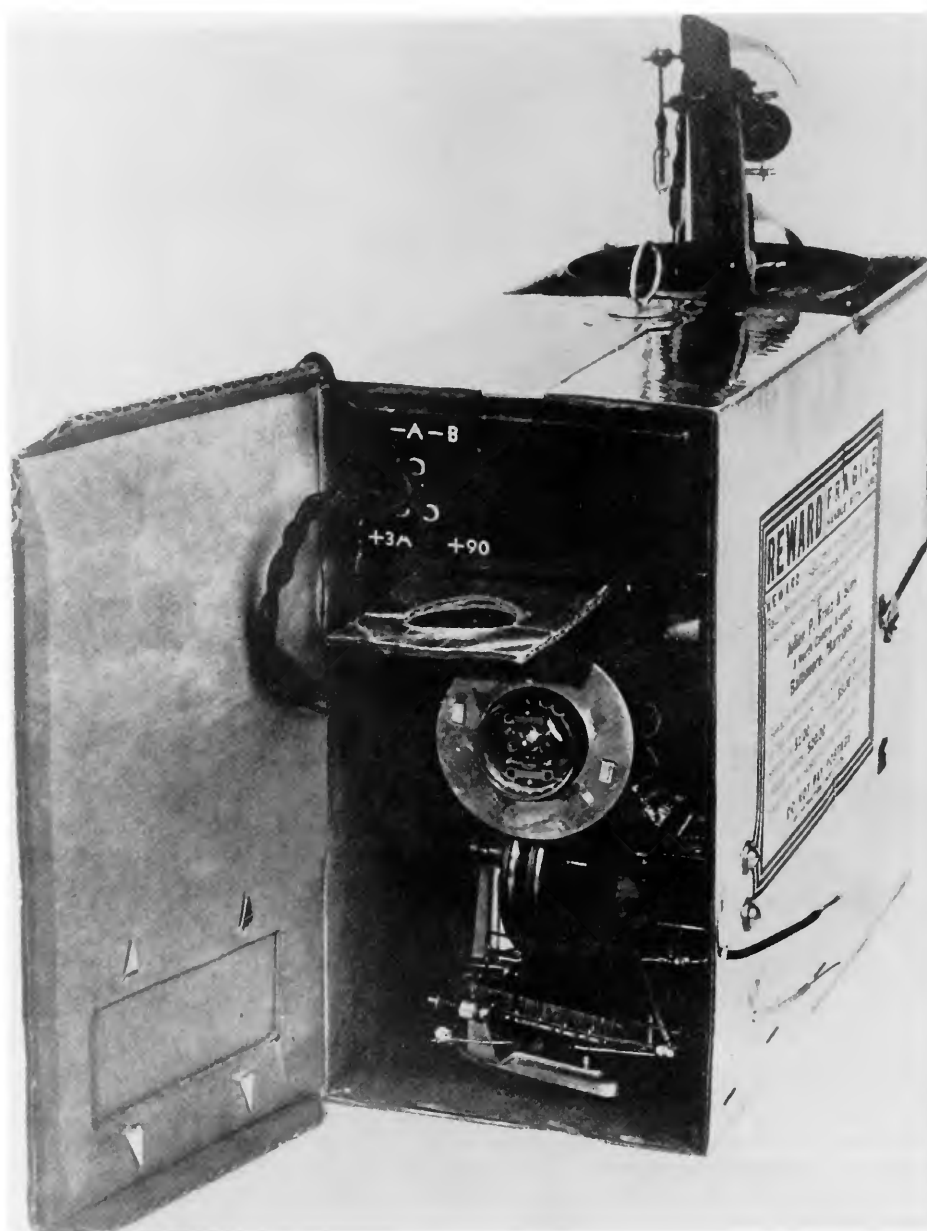
FIGURE 51.—This NBS-Navy radiosonde was manufactured in large quantities by 1940 and incorporated improvements such as an electric hygrometer. The batteries, transmitter, and pressure unit were housed in an insulated box to minimize temperature changes. The temperature tube and electric hygrometer (at rear) were shielded against solar radiation by a double-walled metal tube. The total weight was less than 1 kg; the cost was $25 in 1940. The finder of the balloon after its flight received a monetary award upon return of the radiosonde. (From Snyder and Bragaw, Achievement in Radio , 1986, fig. 52.)
