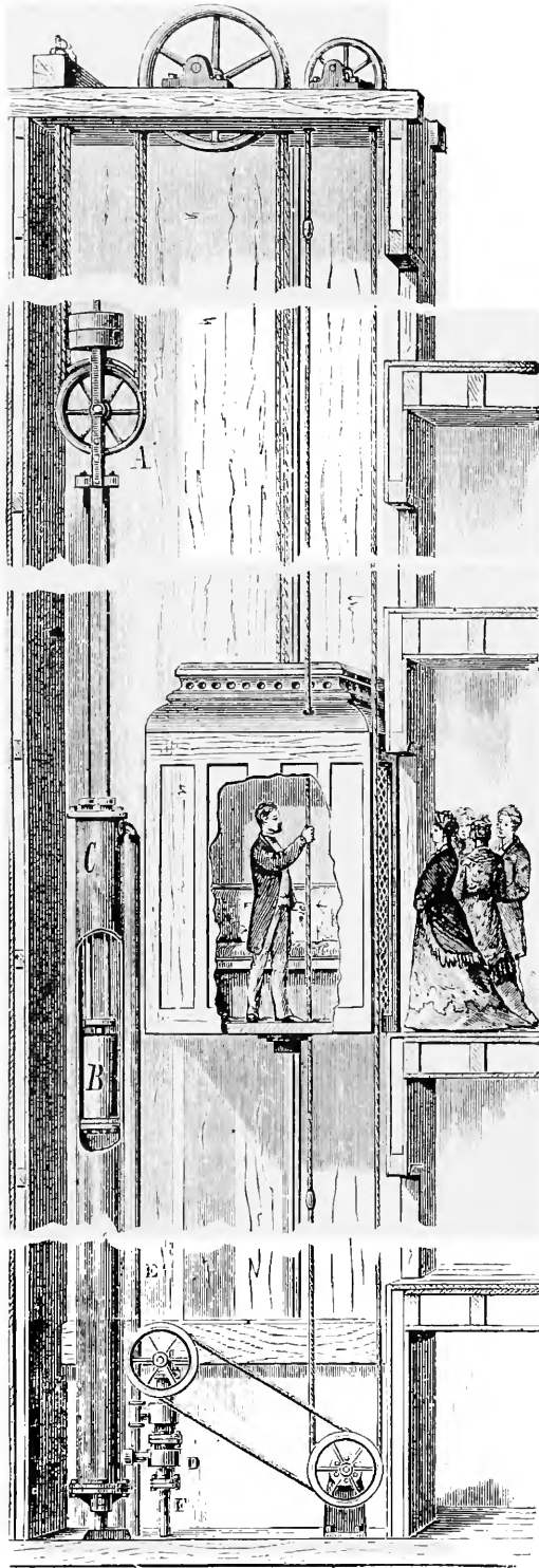
FIGURE 5.—The vertical-cylinder, pulling-type rope-gear hydraulic elevator in its initial mature commercial form, ca. 1875–1880. As in the teagle, control is by endless hand rope, here working the operating or control valve (at the base of the cylinder). For higher rises and speeds the rope was replaced by a lever or crank wheel. Although the basic arrangement was essentially the same for vertical- and horizontal-cylinder machines, with the vertical the dead load of the car was largely counterbalanced by the piston-and-traveling-sheave assembly with only a small amount of additional weight generally being needed. (From The Builder & Wood-Worker [New York], June 1880:iv.)
