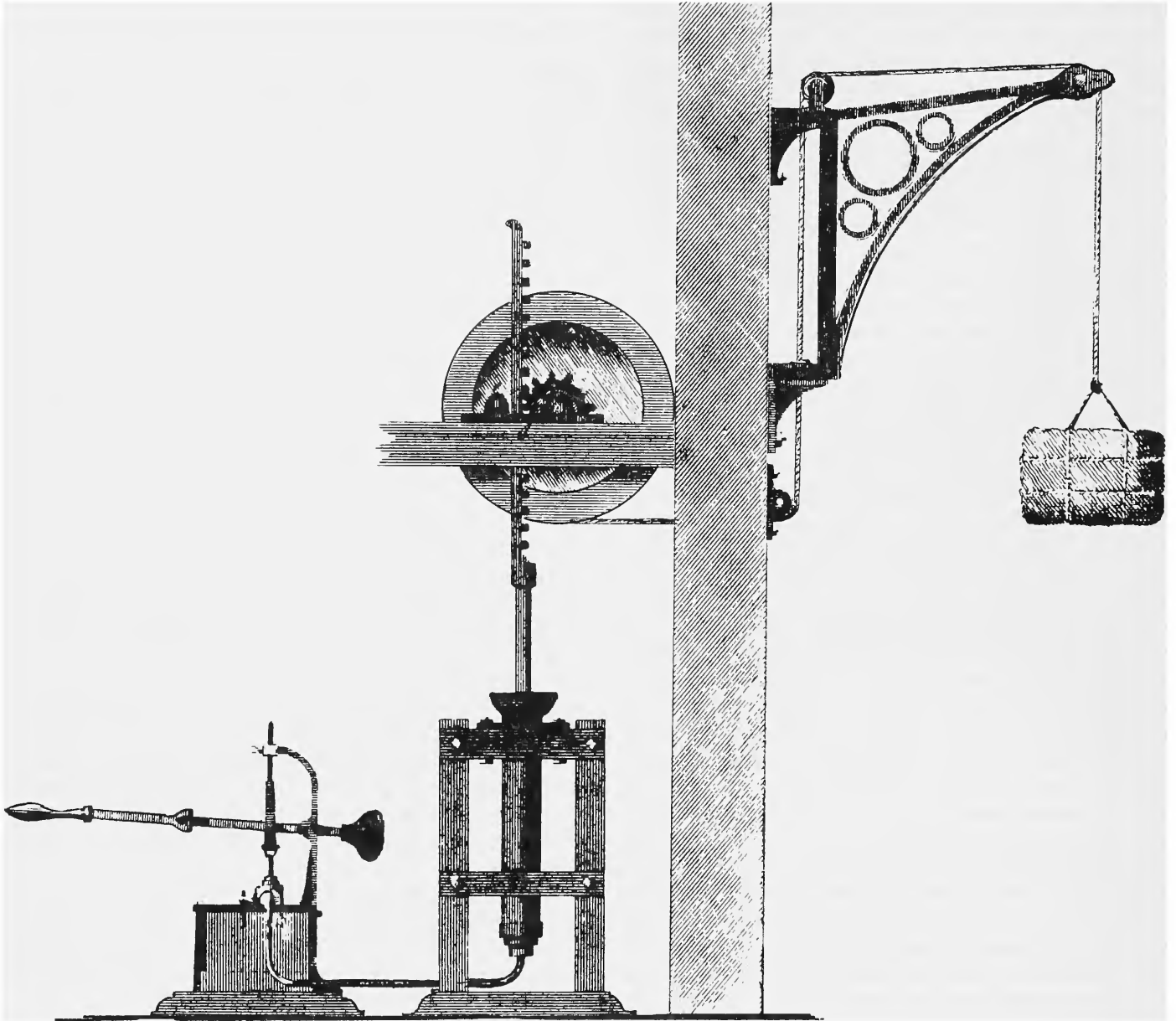
FIGURE 2.—Bramah's adaptation of his basic hydraulic press to the powering of the dock or warehouse crane by introducing a winding drum turned by a rack and pinion. The hydraulic pressure was furnished by a hand pump in most of the few installations mounted by Bramah, the net result being a clumsy and unduly complicated hand crane. (From David Brewster [compiler], The American Edition of the Edinburgh Encyclopaedia [Philadelphia, 1823], plate 215.)
